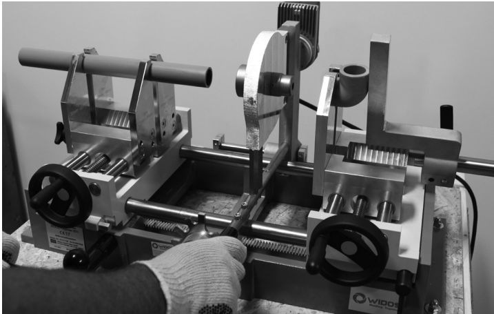
Figure F-8. Move the machine slides with the handle lock to set the heating element into the center between pipe and fitting.
