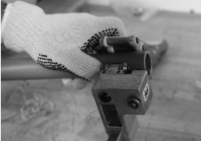
Figure F-17. Remove the outside oxide layer using a scraper. For dimensions larger than 3" (90mm), we recommend using a peeling tool similar to the one shown above for removing the outside oxide layer. Clean the joint surfaces with a purifying agent (e.g. alcohol) and mark the bushing depth.
