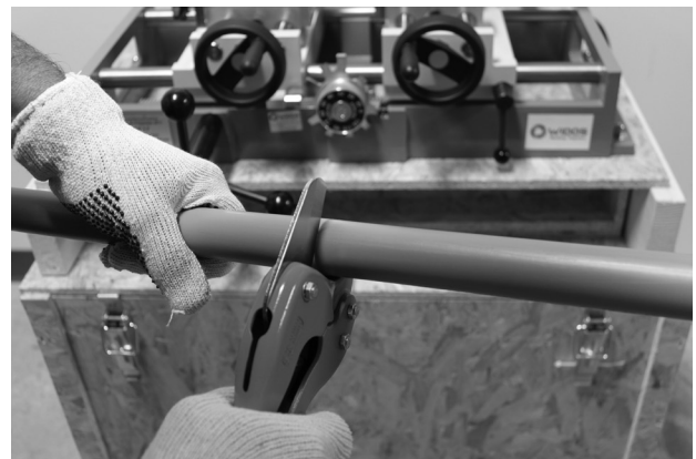
Figure F-1. Measure and cut pipe with suitable pipe cutters to the correct length. Pipe must be squared 90 degrees.
