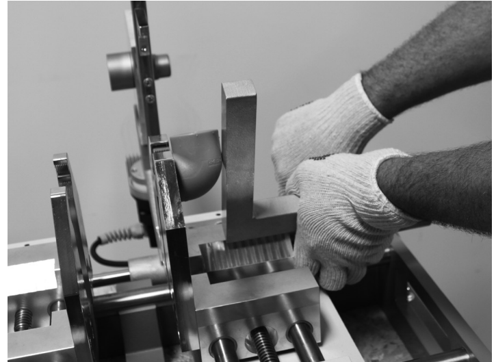
Figure F-6. Place and adjust the fitting in the clamping jaw and adjust the stop to hold the fitting.
