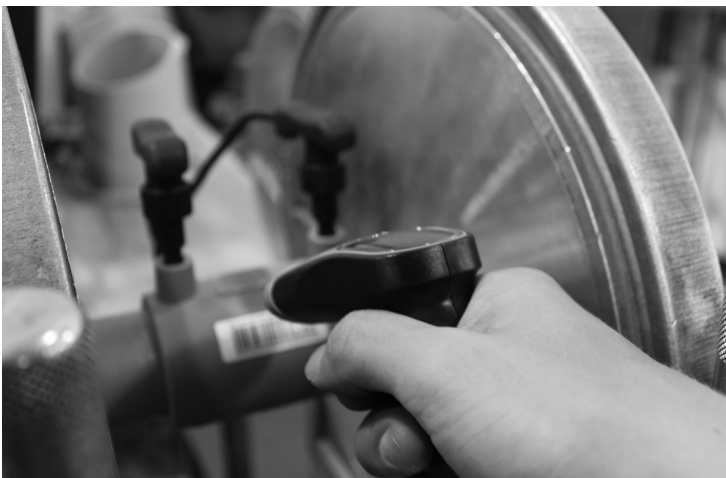
Figure F-21. The welding data can be seen on the bar code label of the socket. The data can also be read by the bar code scanner of the electrofusion machine.
