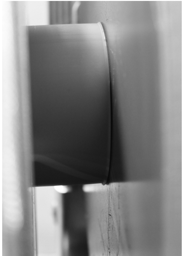
Figure F-14. During butt welding with heating elements, the areas to be joined are heated up to the welding temperature and brought together by prescribed pressure after the heat element has been removed. Heating temperature 410^{\circ}\text{F} (\pm 18^{\circ}\text{F}) .
