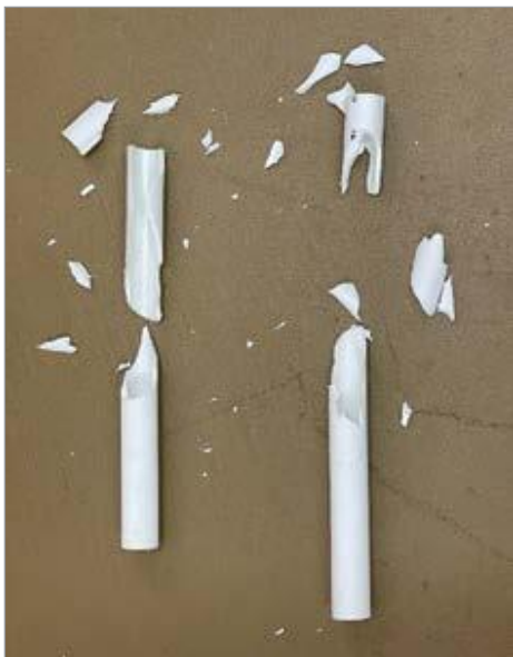
PVC Schedule 40 catastrophic failure mode.
