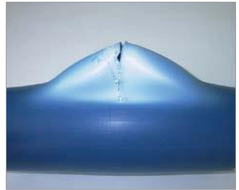
Asahi/America’s Air-Pro® over-pressurized ductile failure in safe mode during burst test (pressure ≥ 800psi).
