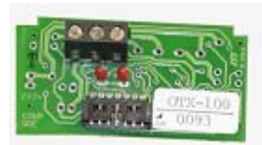
Optional 4-20 mA Transmitter plugs into PCB
